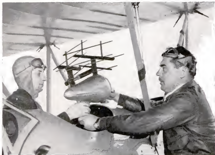
Detector mounted in a plane for a test. It responded to objects fourteen miles away
